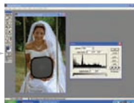
Select the grey dropper and click on the card. The poor exposure and colour balance is automatically corrected. Save these changes as a 'new action'.
